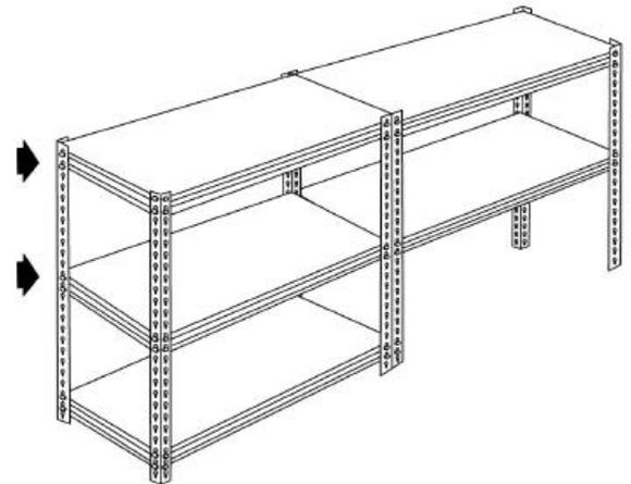
Add a shelf to the previously built level, then continue by adding the fourth and fifth level to the unit using two beams and two braces per level. Tap lightly to properly seat the rivets and add the final shelves to the unit. Install all four end caps to the top of the unit after assembly has been completed (E). Install end caps to post by pressing down on ends.
