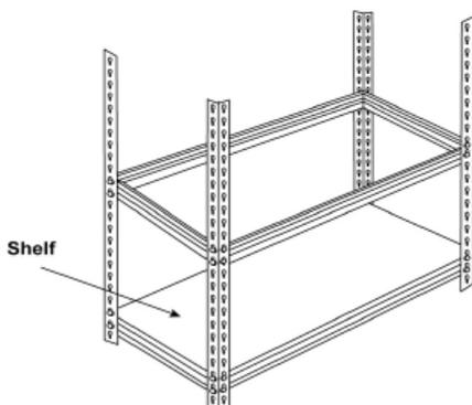
Again place the rivets of the beams and braces into the post slots with the shelf ledge facing up and tap lightly to seat the rivets.
