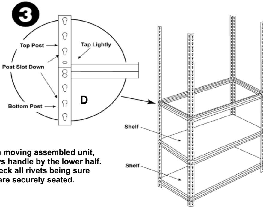
When moving assembled unit, always handle by the lower half. Recheck all rivets being sure they are securely seated.
